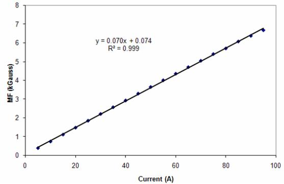
Fig. 2 Dependence of magnetic field on power supply current
