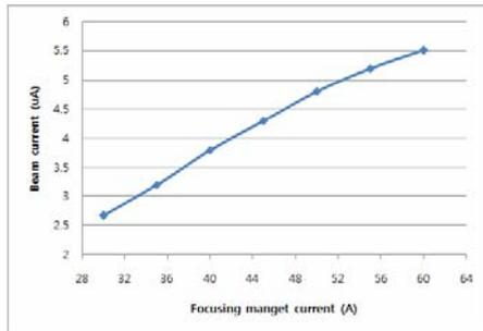
Fig. 5 Dependence of beam current of focusing magnet current.
