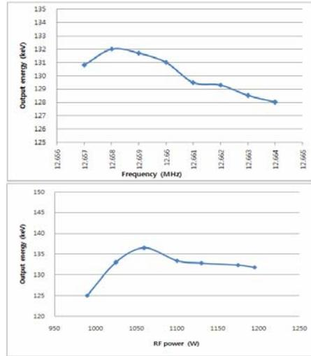
Fig. 6 Output energy versus driving frequency (top) and RF power (bottom)
