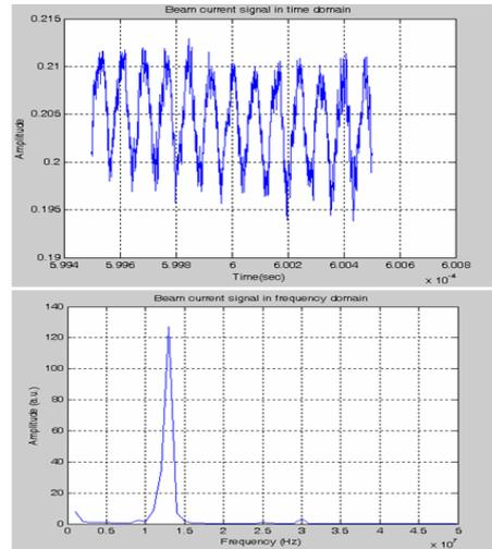
Fig.7 Beam current signal in time (top) and frequency (bottom) domain
