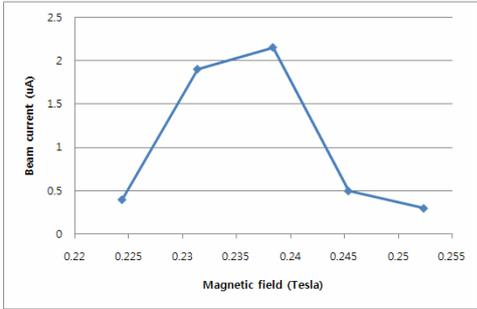
Fig. 4 Accelerated beam current depends on magnetic field (at fix driving frequency of 12.658MHz, rf power of 1.08kW and focusing magnet current of 20A)
