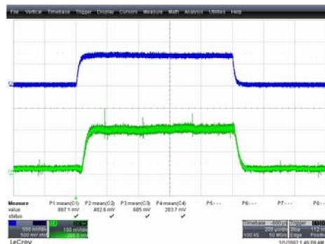
Fig. 3 Wave form of the forward power (C3) and beam current (C4)
